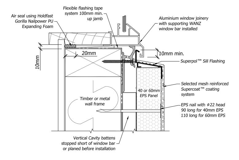
**Note:** In situations where the WANZ window bar is installed at Sill locations, the rear portion of the Superpol<sup>TM</sup> Sill Flashing can be removed and installed on top of the cavity batten allowing the window bar to be fixed suitably
