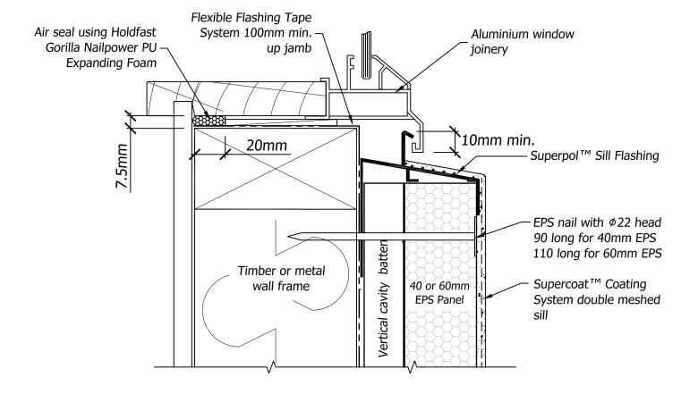
**Note:** In situations where the WANZ window bar is installed at Sill locations, the rear portion of the Superpol™ Sill Flashing can be removed and installed on top of the cavity batten allowing the window bar to be fixed suitably, See Detail SP 6
