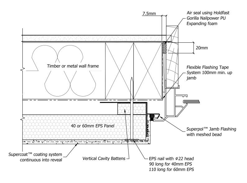
**Note:** Holdfast FIXALL 220LM MS sealant bead between uPVC Jamb Flashing and window joinery to be installed
