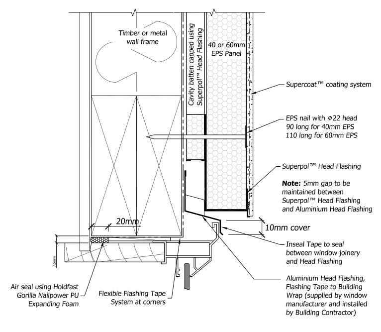
**Note:** Aluminium Head Flashing to be cut and installed flush to window width. Sealing requirements between Superpol Jamb Flashing and Aluminium Head Flashing not shown
