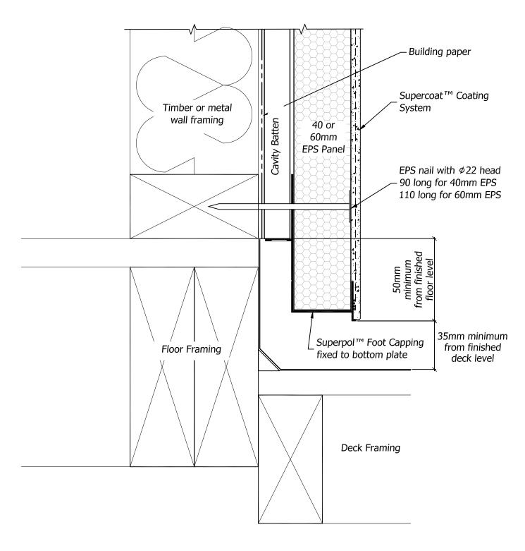
**Note:** Mesh Reinforced Supercoat<sup>™</sup> Tanking Membrane deck lining minimum 150mm upstand. At door openings membrane must return over floor in conjunction with NZBC E2/AS1
