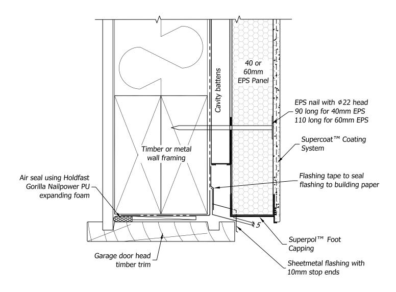
NOTE Above detail is only suitable for standard roller or sectional roller garage doors
