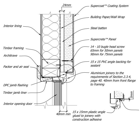
Gap between joinery and Supercoat™ pre-meshed render stop filled with sealant (Holdfast FIX ALL 220LM MS)
