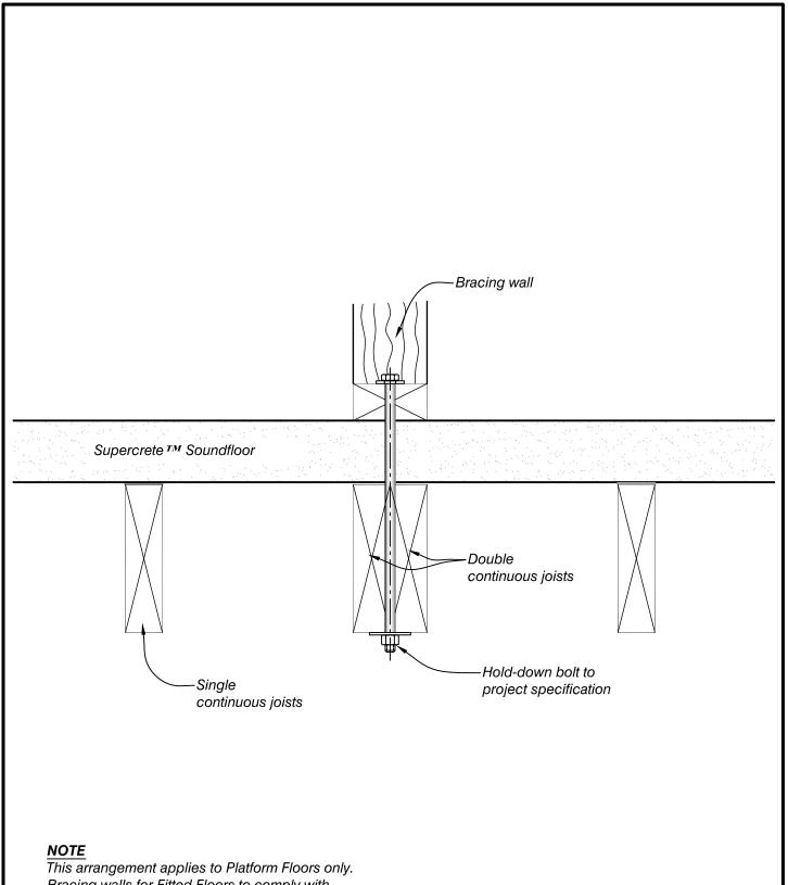
Bracing walls for Fitted Floors to comply with NZS 3604.
