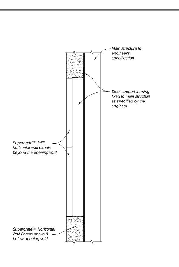
CIWS Horizontal Multiple Panel Width Opening Supercrete Title: Section "A-A" Detail **CIWS CONSTRUCTION**
