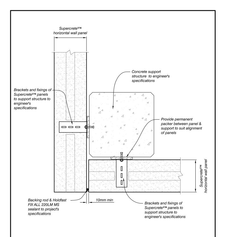
NOTE: For fire rated wall systems, the packer must have the required fire resistance rating, FRR
